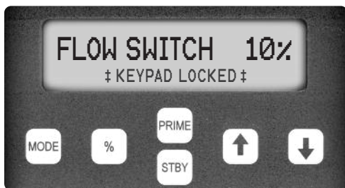
Example of control panel with keypad locked.
