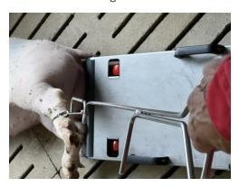
Transporker is stopped with one foot and the user pulls the cadaver onto the platform over the pick-up rollers integrated in the ramp. Using the pull rod, Transporker with the cadaver can now be pulled to the cadaver disposal site.
