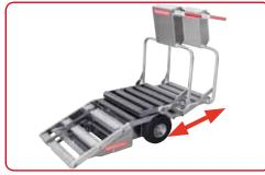
Foldable loading table for working in confined spaces. The user takes the vehicle in retracted state to the animal. The loading table unfolds while pulling the animal onto the vehicle.
