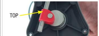
Apply a few drops of Tailwell lubricant to the rotator arm (9) and rotator bearing (8) as well as to the cutters. Refit the top cover and secure it with the six cap screws (11) being careful not to over tighten them.
