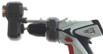
To attach the Tailwell2 tail trimmer to your drill loosen the drill chuck so that the trimmer drive shaft fits fully into the chuck and then tighten.
