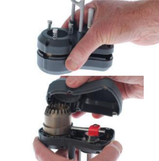
Step 4. The cutters can be removed and separated. You should not have to force them apart. Check for wear and damage.
