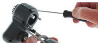
Step 2. Using the hexagon screw driver provided in the kit, undo the six cap screws (11) that secure the top and bottom case together.
