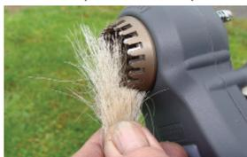
You should be able to turn the driveshaft by hand. You can test the setting with a small amount of tail hair with the drill running.
