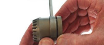
Wash thoroughly to remove all traces of paste. Repeat if necessary to get a smooth cutting action. Wash thoroughly and lubricate before reassembling.
