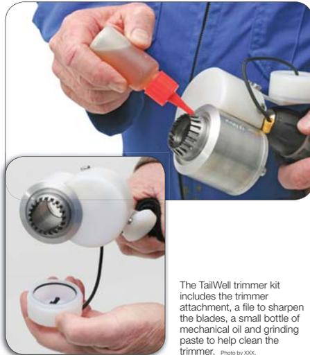
The TailWell trimmer kit includes the trimmer attachment, a file to sharpen the blades, a small bottle of mechanical oil and grinding paste to help clean the trimmer. Photo by XXX.
