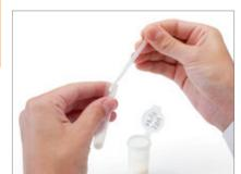
Using pipette, draw up milk to indicator line (450  $\mu$ L  $\pm$ 50  $\mu$ L).† Add milk to sample tube.
