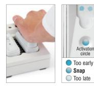
As the edge of the activation circle begins to disappear, press down firmly until you hear a distinct "snap." If activation takes more than 60 seconds, result may be inaccurate.‡
