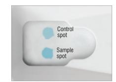
**Negative** Sample spot is darker than or equal to control spot. No drug residue detected.
