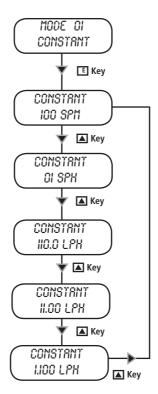
Choose "CONSTANT" working mode: "SPH" (strokes per hour), "SPM" (strokes per minute), "LPH" (litres per hour).
