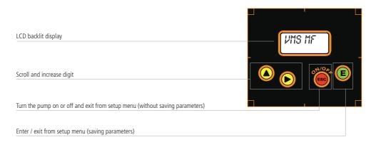
The "VMS MF" pump is equipped with a keyboard. To avoid any misunderstanding during next chapters all keys will be described as shown on this legend:
