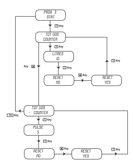
"TOD DOS" means total dosed product since pump last reset. "COUNTER" means strokes numbers since pump last reset.
