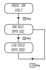
To work in this mode is necessary to specify the "HIV" (maximum working tension), "LOV" (minimum working tension) and "SPM" (strokes per minute) values that pump will produce between the parameters.
