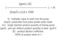
If obtained "N" is < 1 then install a pulse sender water meter that produces less pulses. Otherwise use the "DIVIDE" mode and divice for 1/N. It's also possible to fix the problem trying to decrease product dilution.
