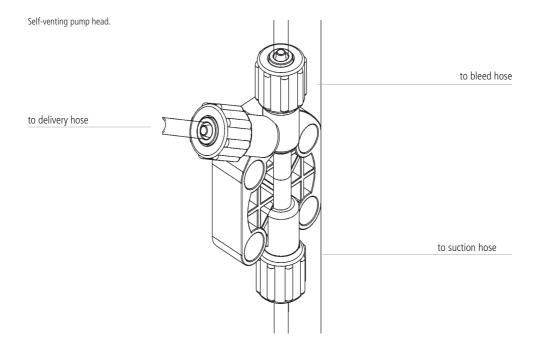
Self-venting pump head must be used when using chemicals that produce gas (i.e. hydrogen peroxide, ammonium, sodium hypoclorite at particular conditions).
