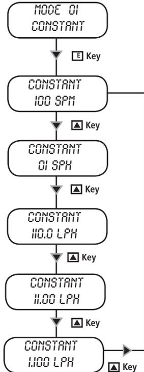
Choose "CONSTANT" working mode: "SPH" (strokes per hour), "SPM" (strokes per minute), "LPH" (litres per hour).
