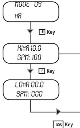
To work in this mode is necessary to specify the "HmA" (maximum working current), "LOmA" (minimum working current) and "SPM" (strokes per minute) values that pump will produce between the parameters.
