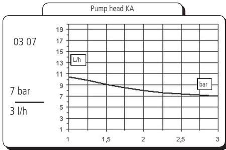
Flow rate indicated is for H<sub>2</sub>O at 20°C at the rated pressure. Dosing accuracy  $\pm 2\%$  at constant pressure  $\pm 0,5$  bar.
