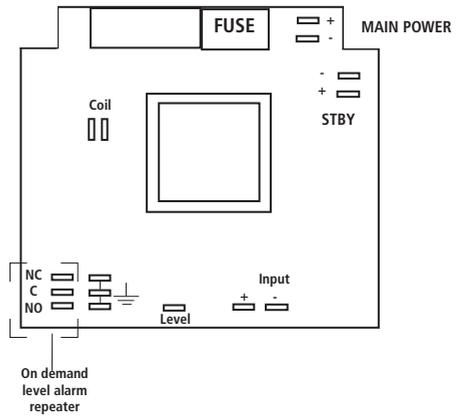
VMS MF FOR WATER METER WITH HALL EFFECT CONNECTION
