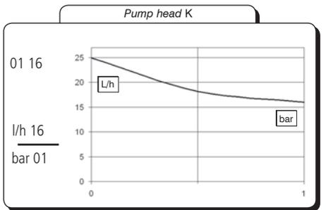
Flow rate indicated is for H<sub>2</sub>O at 20°C at the rated pressure.
