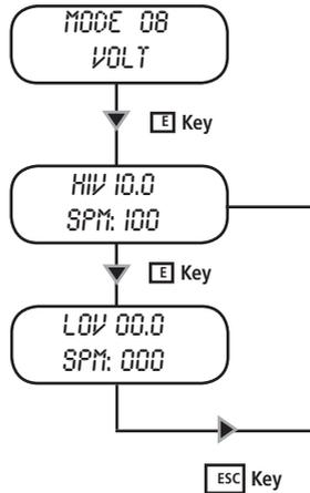
To work in this mode is necessary to specify the "HIV" (maximum working tension), "LOV" (minimum working tension) and "SPM" (strokes per minute) values that pump will produce between the parameters.
