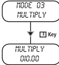
Use this mode if: connected pulse sender water meter produces few pulses and pump must multiply them for correct dosing activities. See formula below to verify this value.
