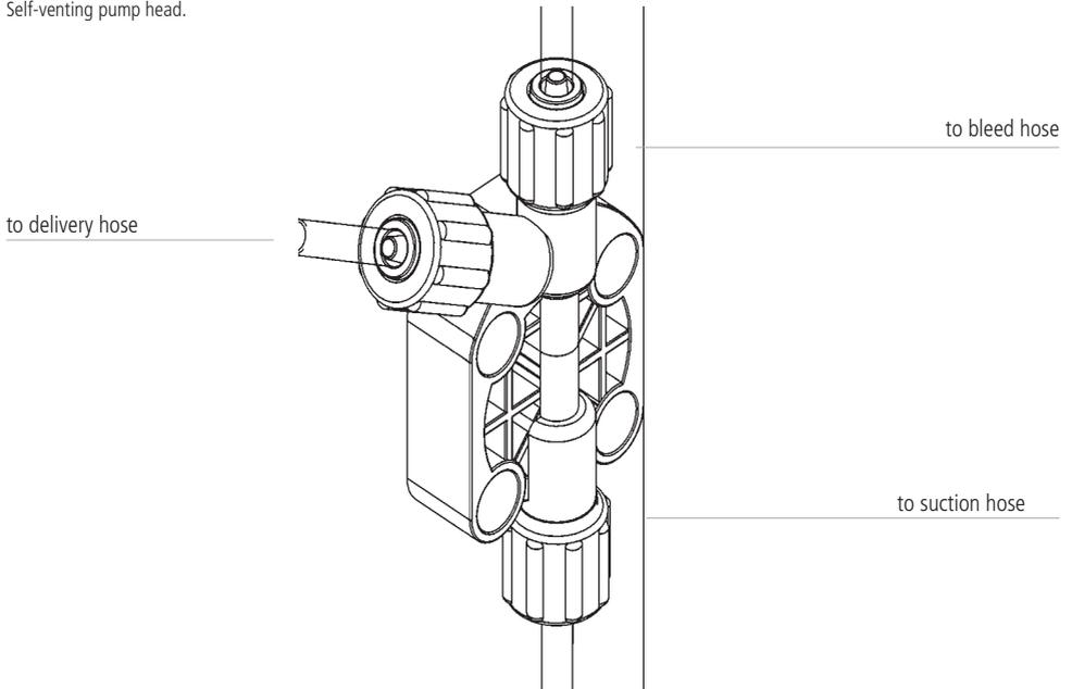
Self-venting pump head must be used when using chemicals that produce gas (i.e. hydrogen peroxide, ammonium, sodium hypochlorite at particular conditions).
