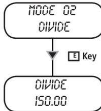
Use this mode if connected pulse sender water meter produces many pulses and pump must divide them for correct dosing activities. See formula below to verify this value.
