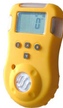
This cell-phone-sized personal gas detector alerts workers to dangerous levels of hydrogen sulfide gas.
