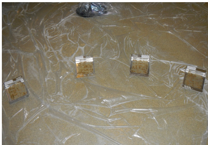
Figure 1. Application of feces to the aluminum coupons. Feces were applied to the coupons using a disposable flat spreader to produce a thin even layer on the floor of the coupon.
