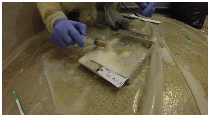
Figure 3. Collection of material from aluminum coupons used to inoculate pigs for the bioassay. A liquid mixture of feces, disinfectant, and saline was aspirated using a 20-mL syringe that was labeled with the pig number of the single pig to be inoculated with the contents from a single coupon.
