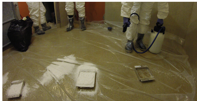
Figure 2. Application of accelerated hydrogen peroxide disinfectant to the aluminum coupons. Disinfectant was applied as a foam using a commercially available 5.7 L pump-up foamer.
