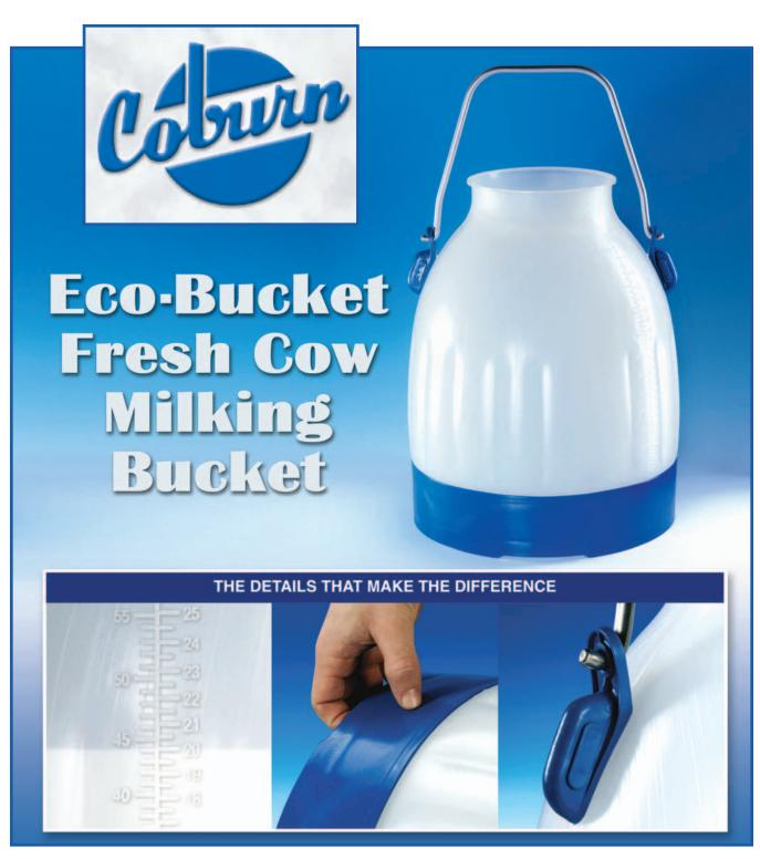
New Eco-Bucket is made of semi-transparent, translucent FDA-approved material. It features smooth seamless molded interior and a reinforcement ring at the bottom for strength and ease of pouring. Eco-Bucket has a stainless steel locking handle, snap-on handle attachment and molded-in permanent scale marked in lbs. and kgs. Bucket capacity is 65 lbs. (30 kgs.)
